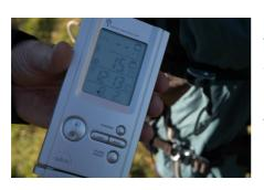
It was held at 2 meters high straight into the wind. The wind speed appeared on the LCD window and the value was recorded on the meteo report form.
