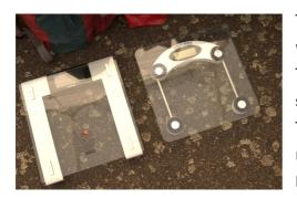
Two normal household balances were used for weighing the pilots and the equipment. They were placed on a firm horizontal flat surface.
