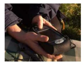
The Compeo and speed probe were made available for the tests by Bräuniger. The compeo is capable of recording time, position, barometric altitude, GPS altitude and true air speed at a rate of 1 Hz. The data is downloadable with the Flychart programme and it is possible to read the produced datafile into Excel for further processing. The user manual can be found at:
