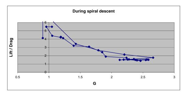
In fact the last graph is the best proof for the relationship between the G-load and the rate of descent. As the G-load increases, the L/D coefficient is decreasing. Because the speed is increasing during the spiral descent, the the sink-rate is increasing even more.
