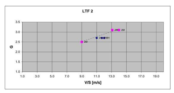
As an extra item I produced a Lift Drag curve from run 2b. I used the vertical speed data derived from the Compeo with Tau=5 [sec].
